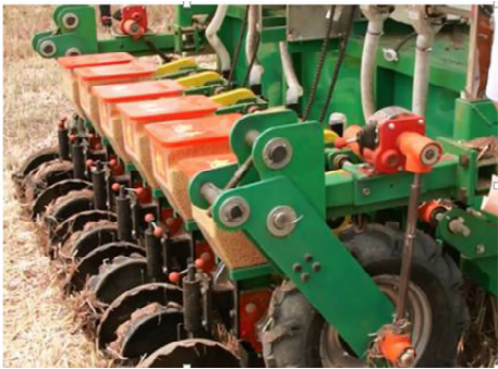
图 3 2BMFJ-6 型麦茬地免耕覆秸施肥播种机 Fig.3 Type 2BMFJ-6 type stubble wheat straw covered no tillage fertilizing and seeding machine
