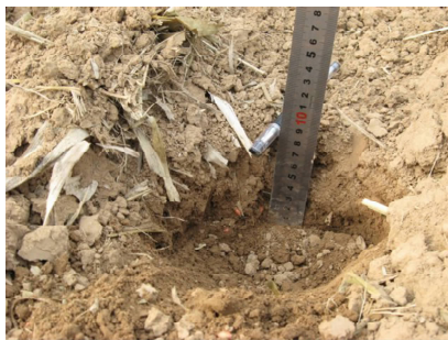
图7 试验地播种深度测定 Fig.7 Experiment of sowing depth determination
