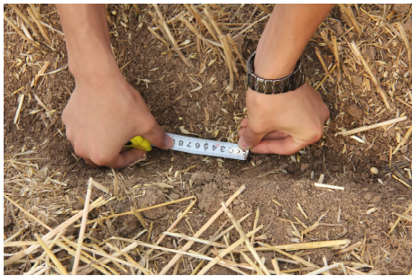
图6 试验地粒距测定情况 Fig.6 Determination of seed spacing
