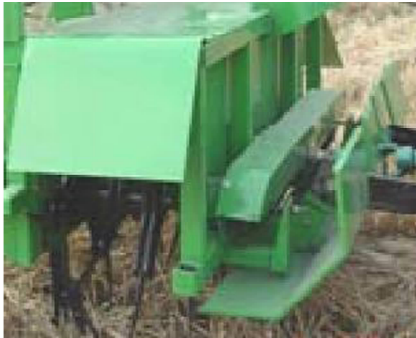
图 4 清秸覆秸装置实物图 Fig.4 Cleaning and covering straw device physical map
