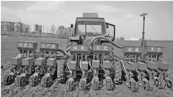
图3 2BPJ-12 型大豆平作密植精密播种机 Fig. 3 2BPJ-12 soybean flat-dense precision seeder
